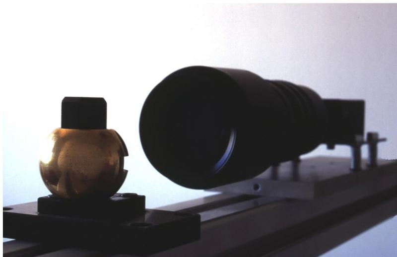
*To check the machining tolerances, SPECIALVIDEO has realized a vision system capable of performing high precision brass balls measurements.*
